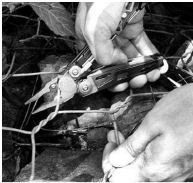
Cutting Fence With Multi-Tool Wire Cutters
