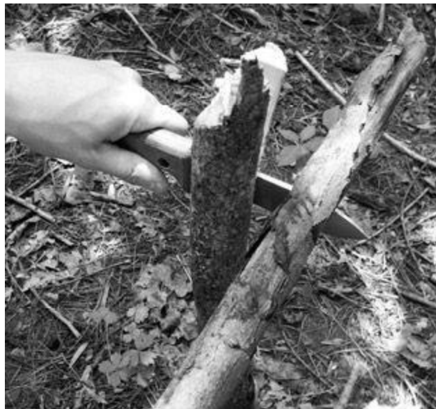
Using Survival Knife to Split Wood (Batoning)
