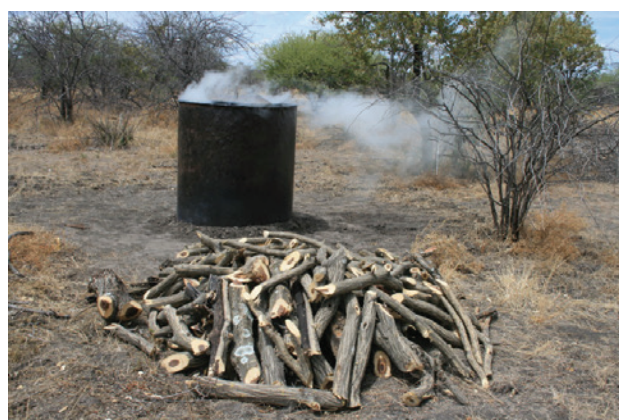
The bush is turned into charcoal by burning it slowly in metal drums.
