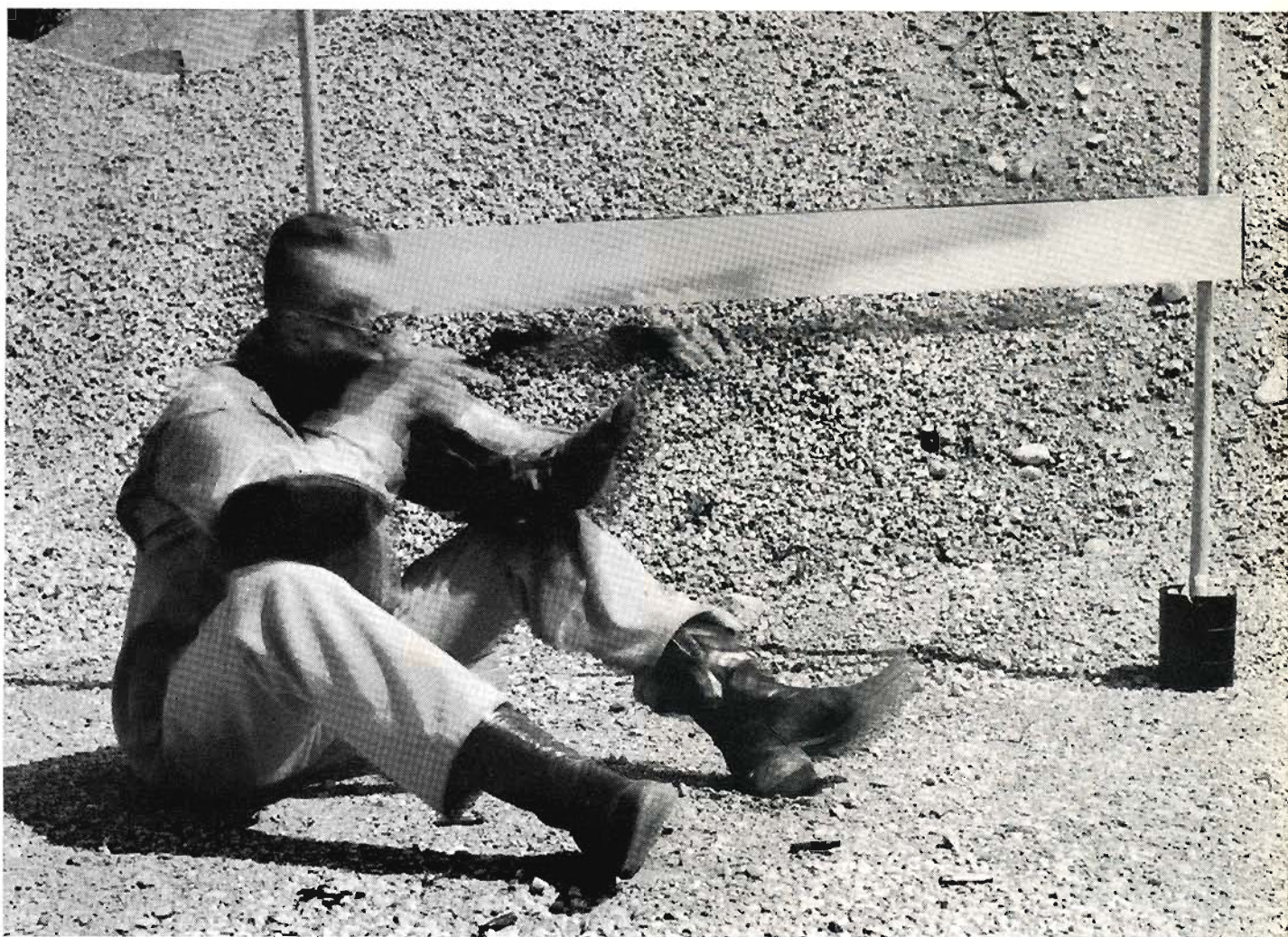
Unbraked Griffin & Howe '06 induced sufficient muzzle rise to lose target from sight completely; amount of muzzle jump is apparent in still photograph. Sha-Cul brake, top opposite page, did well in identical tests.
