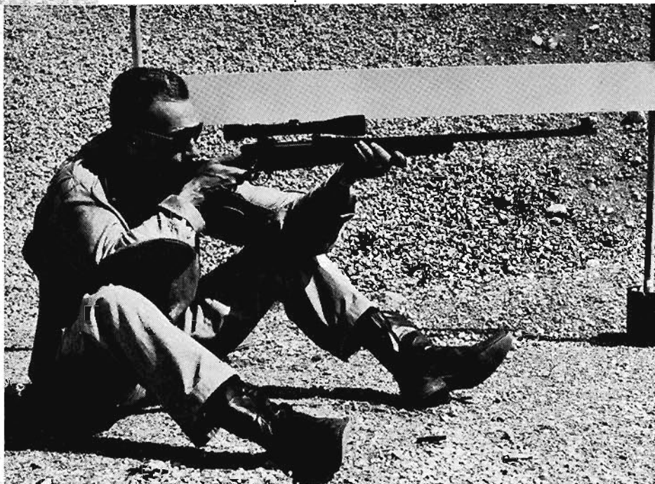
Camera captures muzzle rise which was also recorded on wide, vertical ruler. Picture at right is still photograph, indicating lack of muzzle rise with the Pendleton De-Kicker on Finnbear .30-06.
