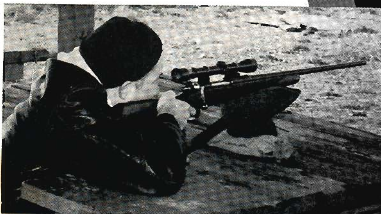
Barrel wear is tested (top) in rifle built by Curry at right. Gann, bottom, shows off .250 Curry Magnum. Gun was fired 8,000 times before it was rebored to caliber .270.
