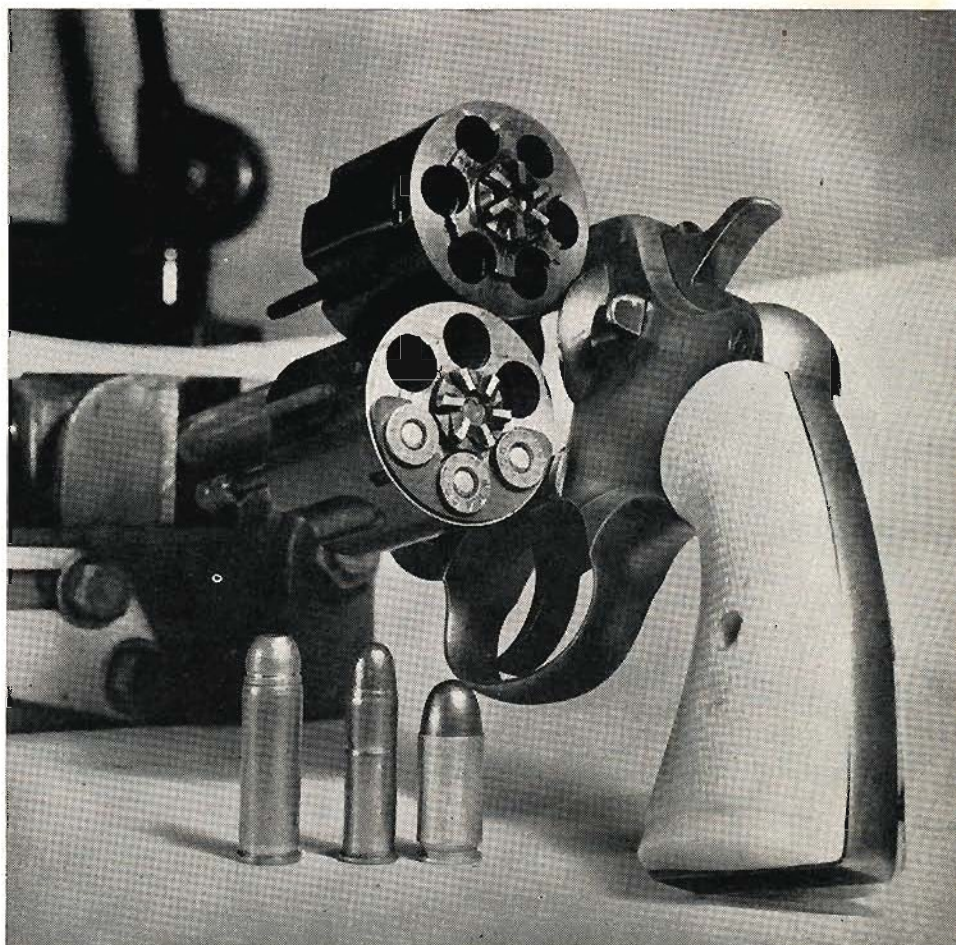
Colt's pawl, ratchet, and ejector assembly with half moon clip that is required to facilitate loading and ejection of the .45 ACP cartridges.
