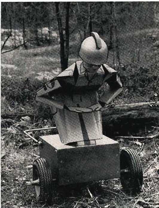
A new, and fully automated, version of the hideous god of war can give even expert riflemen a first class case of jitters. Remote controlled, the motile target dodges, crawls, runs, but collapses when hit by a rifle bullet.
