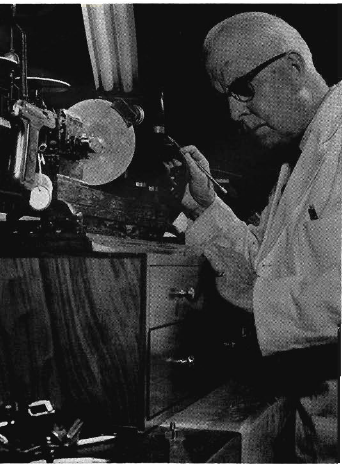
Rifling meter determines angle of rifling in handguns. To make identification of guns more scientific, Mathews invented device himself.
