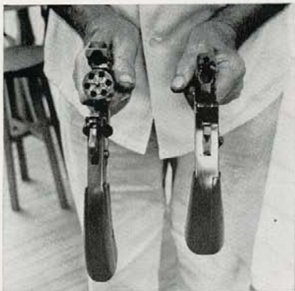
Made to order for trappers, outdoorsmen, gun on left is .22 revolver with .38 barrel, other is chambered for .22 and the .45 Colt cartridge.
