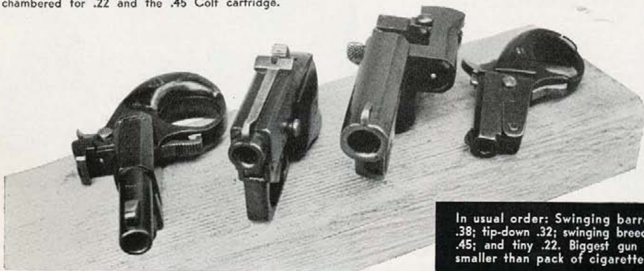
Made to order for trappers, outdoorsmen, gun on left is .22 revolver with .38 barrel, other is chambered for .22 and the .45 Colt cartridge.
