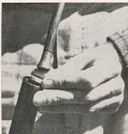
Top wad must sit squarely on shot and must fit bore tightly. If it fits too snugly, it can be notched to let air escape. Put hammer on half cock, seat cap firmly with hammer, fire.
