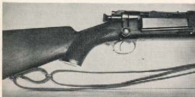
Comb of original Krag carbine stock was raised and a pistol grip added for improved appearance and comfort.
