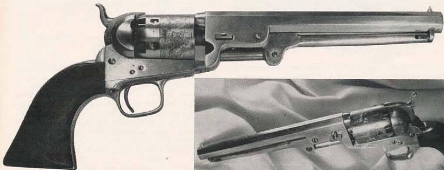
Two views of the author's Navy revolver. Manufactured at Colt's London factory in 1854, it is unique in the absence of any proof marks. This and other odd features lead to theory that it was factory reject.
