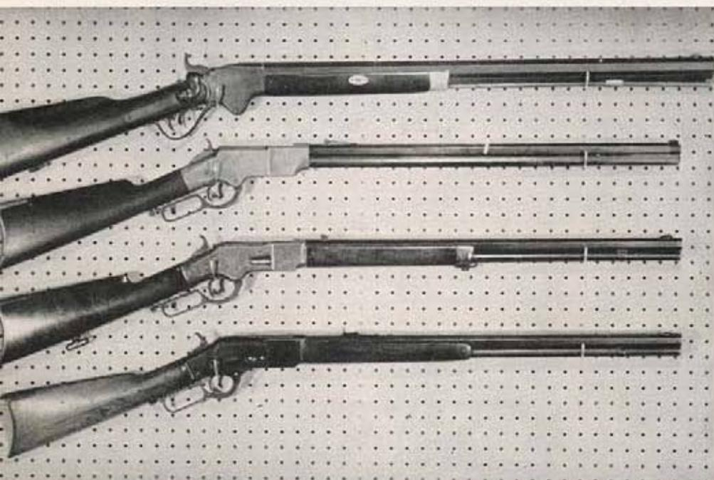
Three guns at top (Spencer, Henry, Winchester Model 66) used rim-fire, not reloadable, ammo. Winchester Model 73 (bottom) handled reloadable ammo, but like guns above, lacked power for long-range buffalo hunting.
