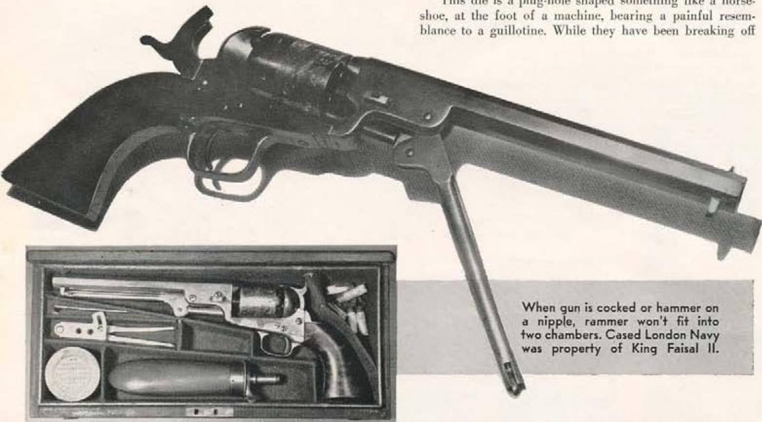
When gun is cocked or hammer on a nipple, rammer won't fit into two chambers. Cased London Navy was property of King Faisal II.
