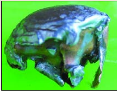
Berger VLDs recovered from the Test Tube retain about 40 percent of their original weight.
