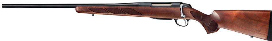
TIKKA T3 HUNTER LEFTHAND based on a totally lefthanded two locking lug T3 action. Bolt features springloaded plunger ejector and it can be easily stripped down for maintenance. Bolt is made of stainless steel.
