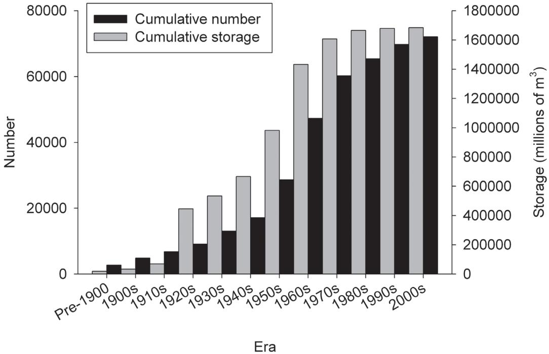
**Figure 4.** Cumulative number of dams and water storage in reservoirs in the United States from before 1900 through 2010. Data from the National Inventory of Dams (USACOE 2009).
