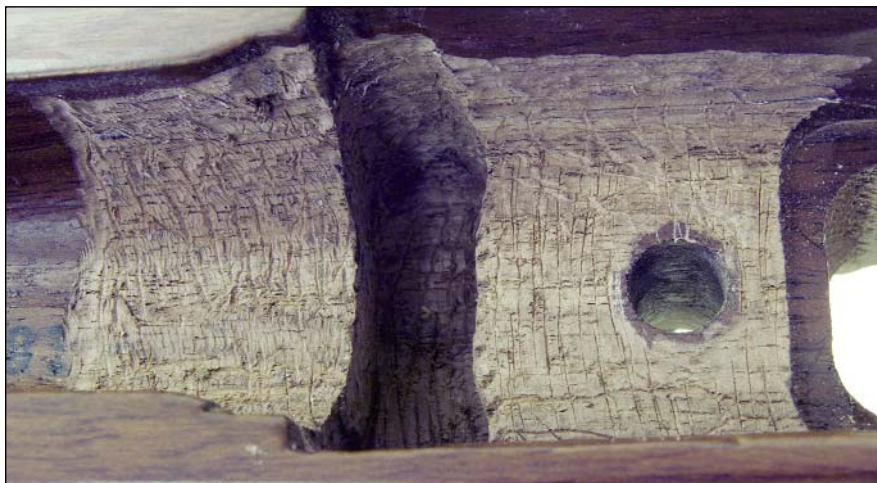
Rough up the receiver ring area before applying glass-bedding compound. The stock must be properly bedded before installing pillars.
