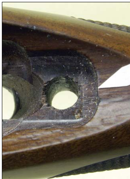
This photo shows the rear tang contact area of the Model 70 stock.
