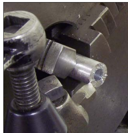
Bedding pillars are easily made on a metal lathe, or they can be purchased.
