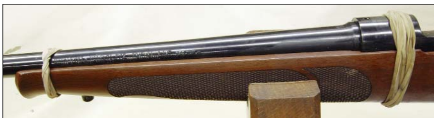
Rubber bands hold the barreled receiver in the stock when glass bedding. Placement here is for bedding the rear tang area.
