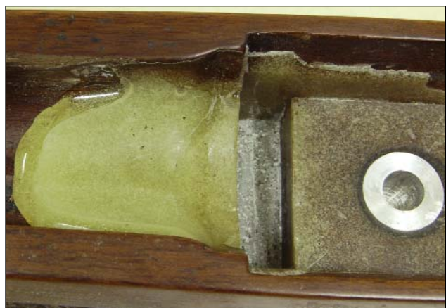
The solid fiberglass bedding pad is shown under the first one inch of the barrel. This is standard bedding procedure.
