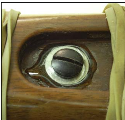
Epoxy has been poured into the recess area around the pillar.
