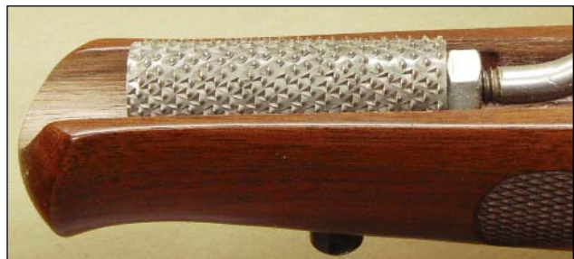
After all other work is completed, the bedding pad is rasped out at the forend tip to free float the barrel.
