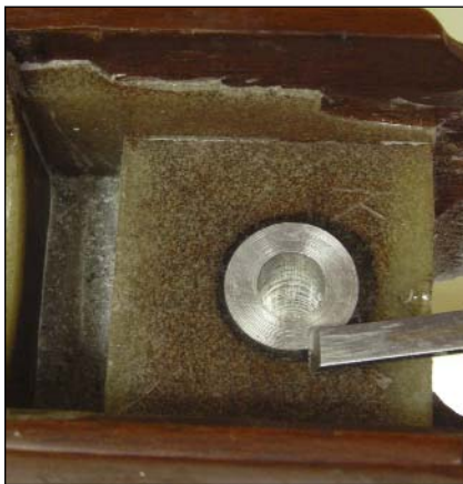
When epoxy cures, the pillar is flush with the bottom of the receiver. No work is necessary here.
