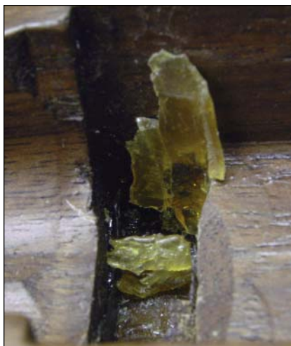
This hot glue-like material was picked out of the recoil lug area of the Model 70 stock.
