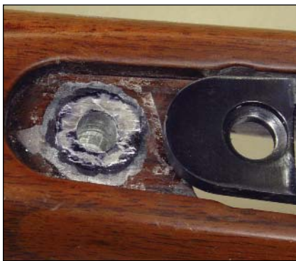
The bottom of the pillar is now cut down to provide a perfect fit with the floorplate tang. This gives solid metal-to-metal contact between the receiver and the bottom metal.
