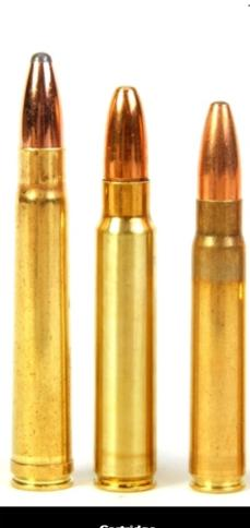
L-R, .375 H&H, .375 Ruger and the gun's original 9.3x62mm. The Ruger, shorter than the .375 H&H, actually has greater capacity because the case head diameter is as large as the belt on the H&H case. The .30-06 Springfield is noted in reference to the medium size action that can accommodate the .375 Ruger, in comparison to the magnum length action required for the .375 H&H.
