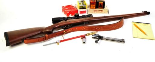
New guns, even with familiar chambers, require requalification of all handloads. Free bores vary, twist rates and chamber differences all contribute to different pressure and accuracy results. Our earlier .375 Ruger handloads were based on the Ruger Hawkeye African with a 23" barrel, rather than the 20" barrel Alaskan. Our modified CZ 550 FS has a 20.5" barrel, but with the same 12" twist as the Ruger models in this chamber, so we had no idea what to expect.
