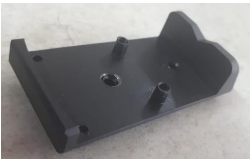
The Steel base which doesn't look as clumsy as the aluminium test base
